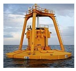
The rising and falling of the waves causes the buoy to move freely up and down. The resultant mechanical stroking is converted via a power take-off to drive an electrical generator. The generated power is transmitted ashore via an underwater power cable
